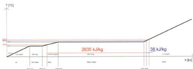
Fig. 4: Temperature-enthalpy diagram of water. Most of the energy is required for the enthalpy of vaporization.
