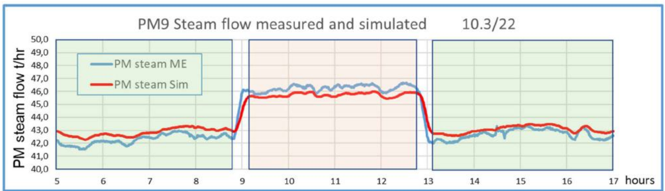
Figure 11. PM9 Steam flow measured and simulated 10 March 2022 during demonstration period (blue highlighted in previous figure)
